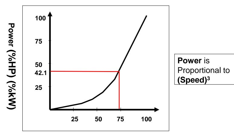
Speed (%RPM), Flow (%GPM)
