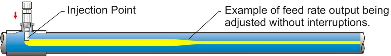
Continuous injection at low motor speed
